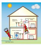
It doesn't matter where you install you LP unit as long as it is on the COLD mains pipe.
