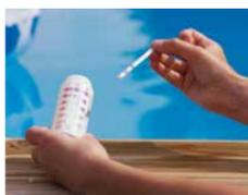
When you decide to purchase a test kit, it is important to choose one that is compatible with the method of treatment you are using: there is one suitable for treatment using bromine and one suitable for treatment using chlorine.
